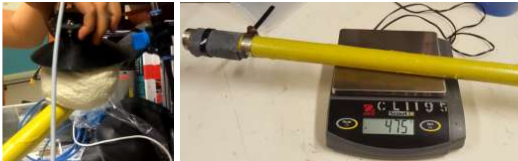
Figure 24: Left - End-effector lifting up a PVC pipe structure of weight 475g, Right - Weight of PVC pipe structure
