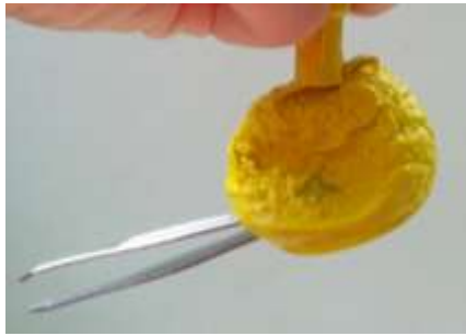
Figure 78: Left - Fine Grain Coffee used to pick up a tweezer by the flat side, Right - Mixture of Fine & Coarse Grain Coffee used to pick up a tweezer by the flat side
