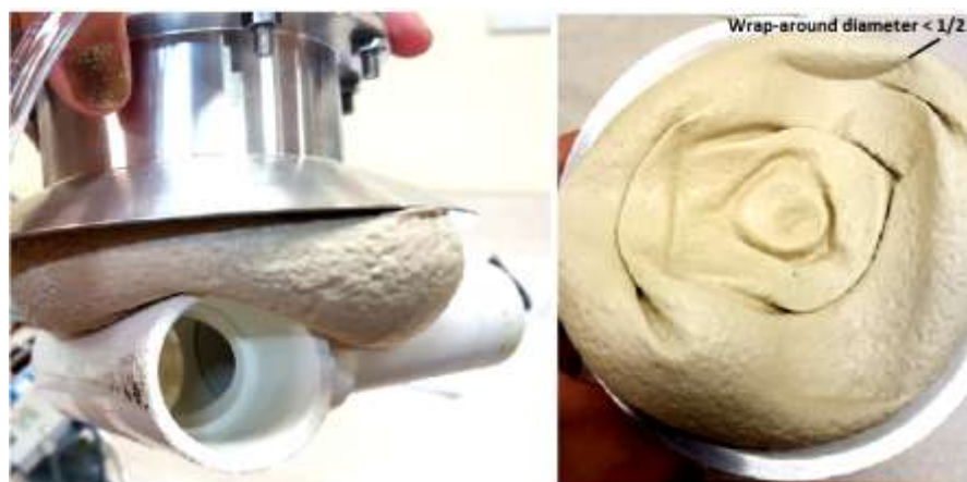
Figure 28: 80% Gripping Success Case from Geometric Interlocking with \frac{1}{2} or less wrap-around Diameter
