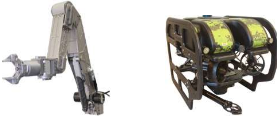
Figure 2: Industry Underwater Manipulators; Left - Schilling Robotics TITAN 4 (FMC Technologies, 2015), Right- Seabotix Grabber on Remotely Operated Vehicle (Seabotix, 2015)
