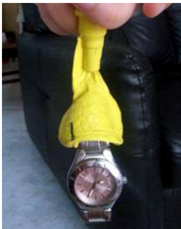
Figure 80: Left - Fine Grain Coffee used to pick up a watch, Centre - Coarse Grain Coffee used to pick up a watch, Right - A mixture of Fine & Coarse Grain Coffee used to pick up a watch
