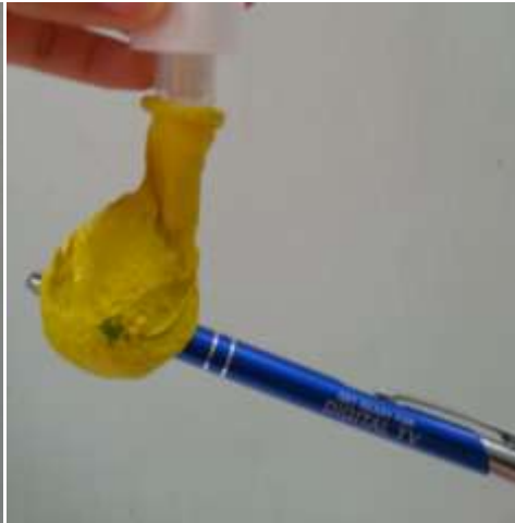
Figure 79: Left - Fine Grain Coffee used to pick up a pen by the cylindrical end, Centre - Coarse Grain Coffee used to pick up a pen by the cylindrical end, Right - Fine Grain Coffee used to pick up a pen from a bucket of water by the cylindrical end
