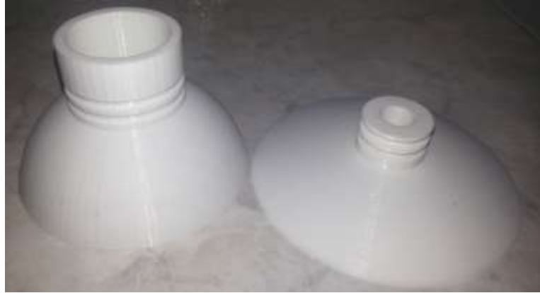
Figure 16: 3-D printed prototypes of Gripping cups - Deep cup versus Shallow wide cup
