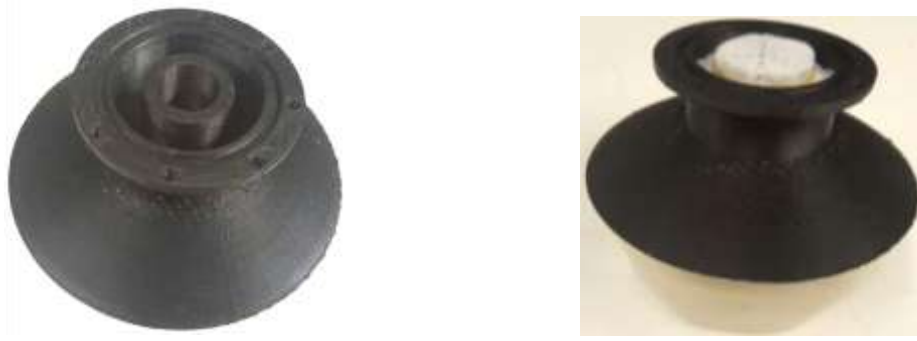
Figure 23: Left - 3-D Printed ABS Prototype of Design 2 End-Effector, Right - End-effector Assembly comprising 3D printed Gripping Collar, Latex Balloon, Coffee Powder and Filter Paper
