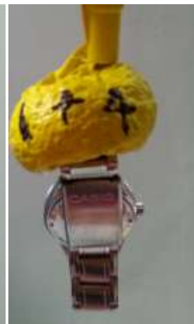
Figure 80: Left - Fine Grain Coffee used to pick up a watch, Centre - Coarse Grain Coffee used to pick up a watch, Right - A mixture of Fine & Coarse Grain Coffee used to pick up a watch
