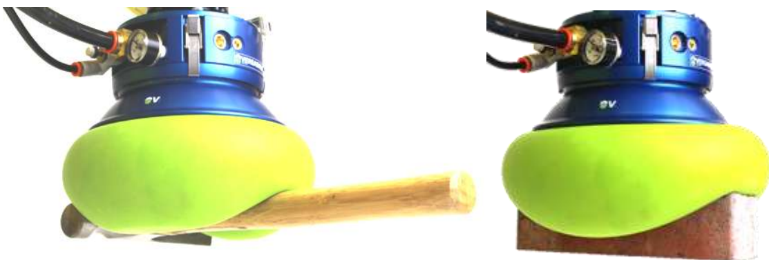
Figure 7: Empire Robotics' VERSABALL Gripper Conforming to Shape and Lifting Objects; Left - Hammer, Right - Brick, (Empire Robotics, 2016)
