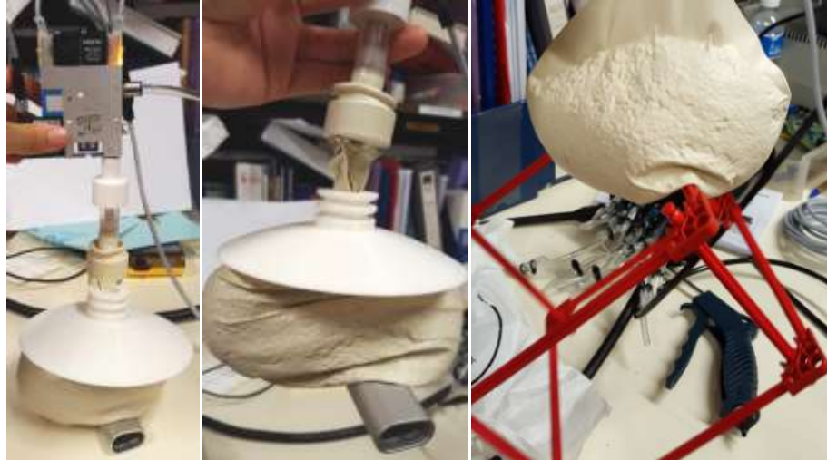
Figure 18: Left - Vacuum Pump is connected to the 24" gripper via Custom-made adaptor, Centre - Jamming Gripper is successful in picking up the oval metal structure, Right - Jamming Gripper is successful in picking up the K'nex
