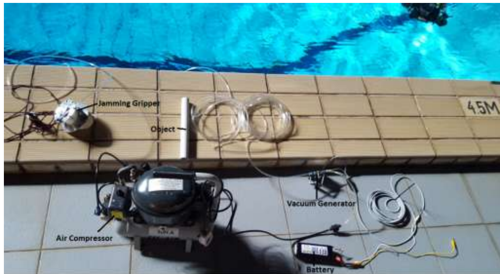
Figure 30: Experimental Setup for testing Jamming Gripper in Water
