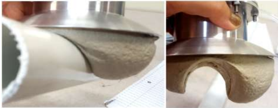
Figure 29: 20% gripping success case, Left– Gripper does not contact ground (Round underneath), Right - \frac{1}{2} or less wrap-around Diameter
