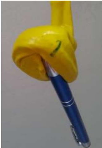
Figure 79: Left - Fine Grain Coffee used to pick up a pen by the cylindrical end, Centre - Coarse Grain Coffee used to pick up a pen by the cylindrical end, Right - Fine Grain Coffee used to pick up a pen from a bucket of water by the cylindrical end
