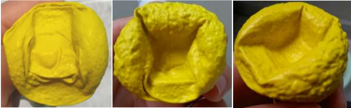
Figure 14: Left – Fine Grain Coffee leaving relatively Less Defined Imprint on membrane, Centre - Coarse Grain Coffee leaving relatively More Defined Imprint on membrane, Right – Fine & Coarse Grain Mix leaving relatively More Defined Imprint on membrane
