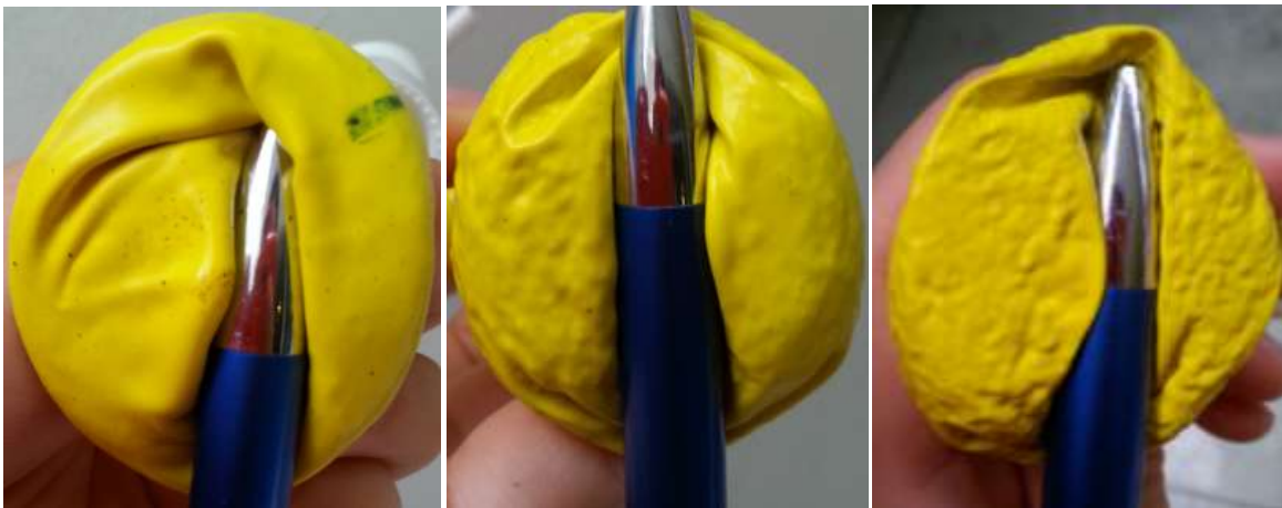
Figure 13: Left - Fine Grain Coffee enables relatively higher object conformation, Centre – Coarse coffee enables relatively lower object conformation, Right – Fine & Coarse Grain Mix enables relatively higher object conformation
