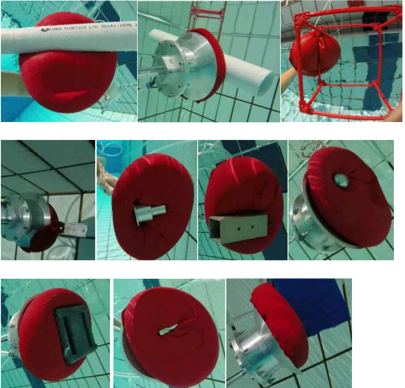
Figure 84: Gripping of Various Objects in air trials; First row (from left) – 25mm PVC Pipe, 43mm PVC Pipe, K'nex Structure, Second Row (from Left): U channel, Odd Geometric Structure, Square tube, Sphere ,Third Row (from left): 2 Pearl Weight, Screwdriver Head, Kick Board
