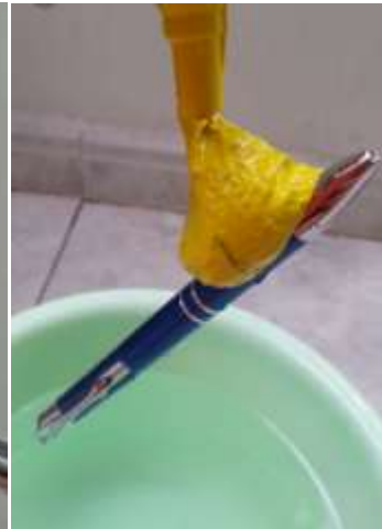
Figure 79: Left - Fine Grain Coffee used to pick up a pen by the cylindrical end, Centre - Coarse Grain Coffee used to pick up a pen by the cylindrical end, Right - Fine Grain Coffee used to pick up a pen from a bucket of water by the cylindrical end
