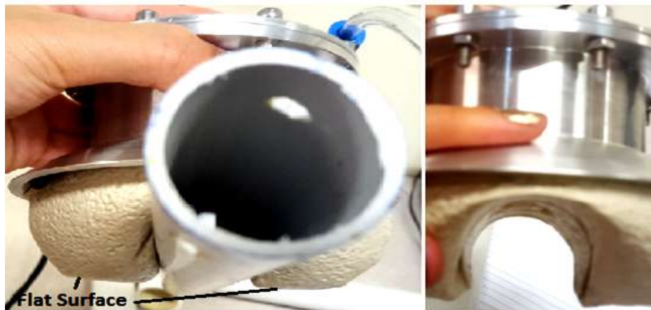
Figure 27: 100% gripping success case, Left – Gripper contacts ground (Flat underneath), Right - \frac{3}{4} or more wrap-around Diameter
