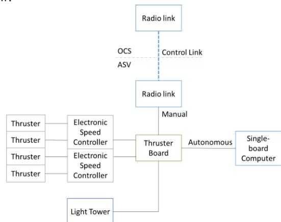
Figure 3. ASV Propulsion System Overview
