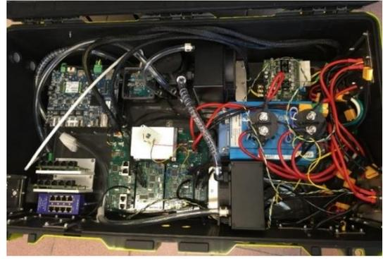
Figure 7. Cable Assembly in ASV main hull
