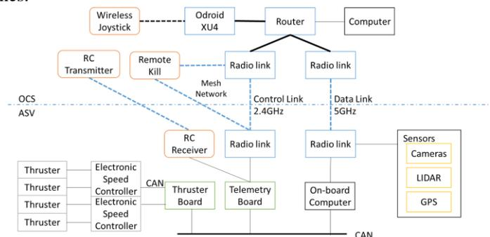
Figure 4. Wireless communication system between OCS and ASV
