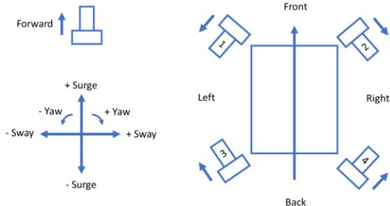
Figure 8. Thruster direction & thrust vector resolution
