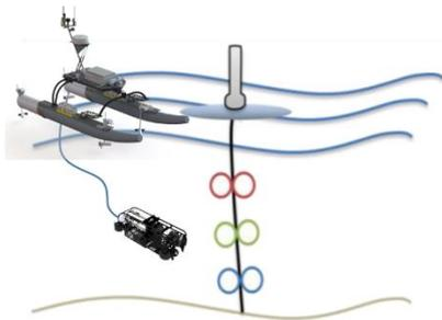
Figure 1. AUV deployment for underwater mission by ASV
