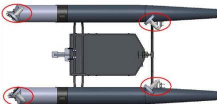
Figure 2. Thruster Layout on the WAM-V vessel (bottom view)
