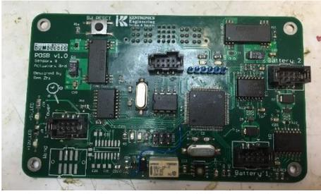
Figure 5. Fully populated ASV thruster board
