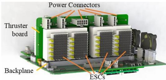
Figure 6. 3D Placement of AUV Thruster Board with ESCs and backplane
