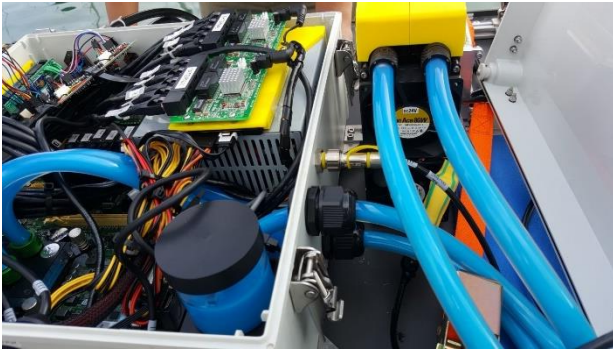
Figure 3. Overview of the Cooling System
