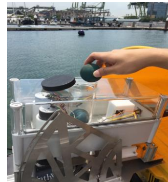
Figure 5: Loading of balls into BBASV 2.0 Ball Shooter
