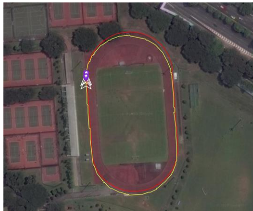
Figure 31: Field test with GNSS receivers (SBG Ellipse-N in red line and Novatel OEM628 in yellow)
