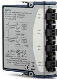
Figure 10: NI9223 Analog Input Module from National Instruments
