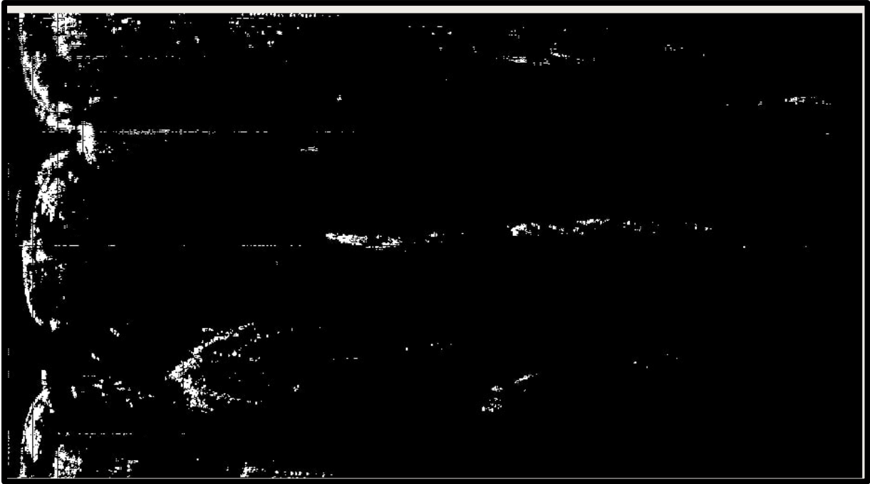
Figure 11: Raw radar polar image with noise, vertical axis represents yaw from 0 to 2\pi , horizontal axis represents range from 0m to 1500m
