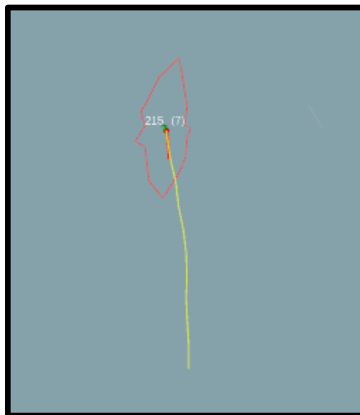
Figure 17: Sample radar track with cluster outline (in red), previous track motion (yellow path) and the unique track id (white text)
