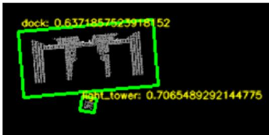
Fig. 9: LiDAR BEV detection (in simulation).
