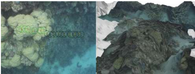
Fig. 2: 3D map generation using sonar and camera on the Great Barrier Reef
